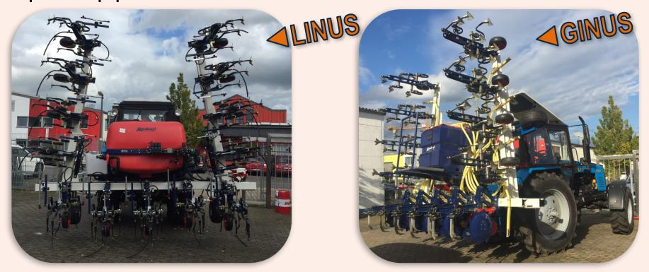
The GELIO cultivator can optionally be equipped with the LINUS system for input of liquid fractions in the inter-row or in the row, as well as on the leaf surface. The system GINUS can be used for input of granular fertilizers in the inter-row or under the sweeps during the cultivating.
