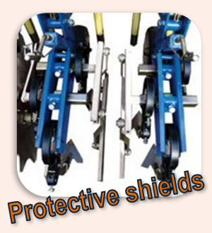
Protective shields protect the plants from undercutting.
